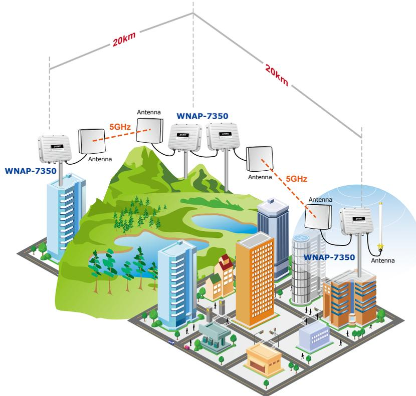
With two built-in N-type antenna connectors, the WNAP-7350 brings higher coverage and longer distance of wireless connection. The WNAP-7350 provides high output power with multiple adjustable Tx controller, which allows CPE users to easily install and adjust the suitable value in appropriate locations. The WISP mode supported in the WNAP-7350 also enables CPE users to connect to Internet via local WISP provider conveniently.
