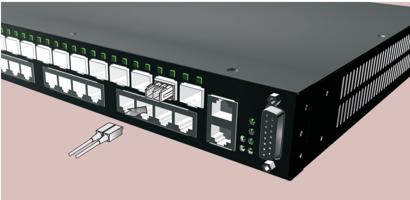
Figure 16: Making Connections to SFP Transceivers
