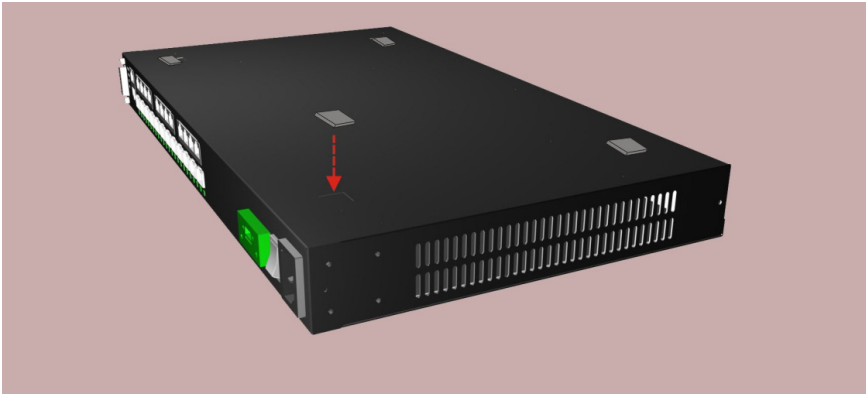
Figure 7: Attaching the Adhesive Feet
