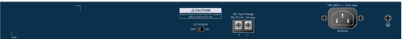
Figure 2-1-38: Rear Panel of GS-4210-24T4SR
